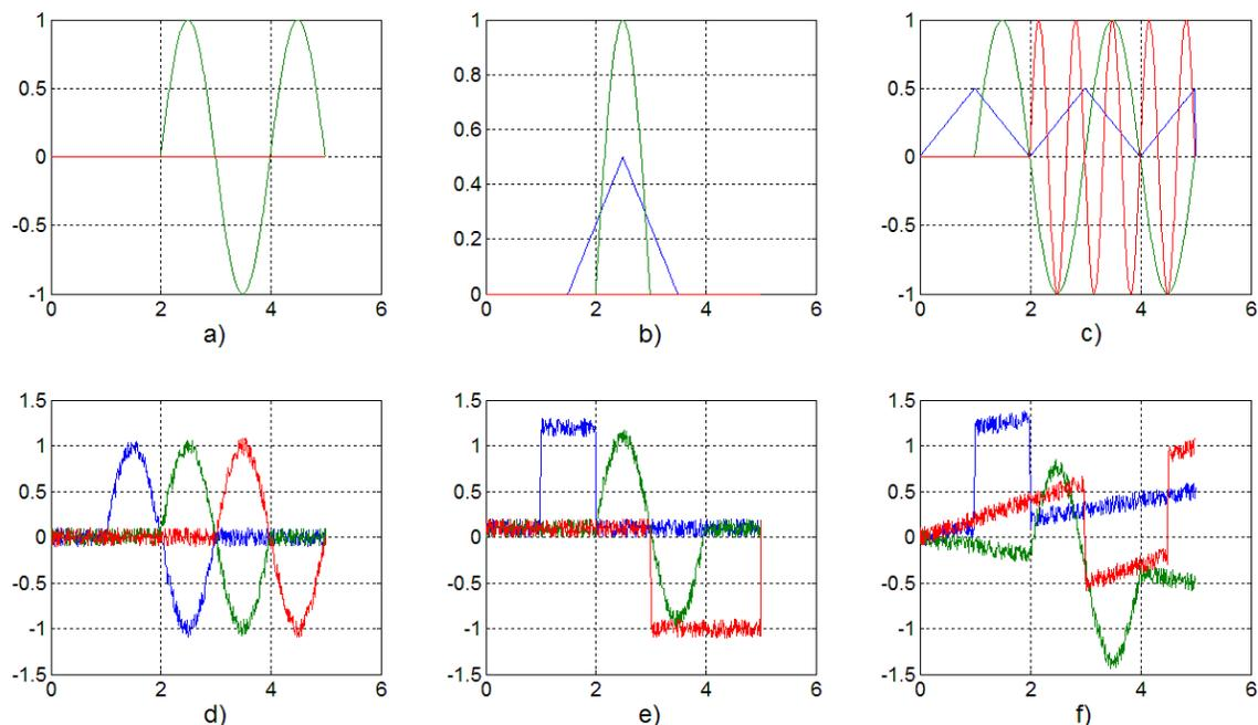
**Figure 2.** Generated gyros data (turn rate versus time): a) simple 1D rotation; b) overlapping rotations around two axes; c) overlapping rotation around all axes with different intensity; d) noised 3D overlapping rotations; e) noised 2D overlapping rotations with bias; f) noised 2D overlapping rotations with different trends
