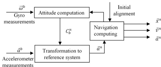
**Figure 1.** Functional diagram of strapdown navigation system
