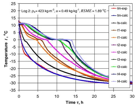
**Figure 2.** Calculated and experimentally determined change in  $t_m$ ,  $t_s$ , and  $t$  in 4 points of the Log 2 during its 30 h freezing
