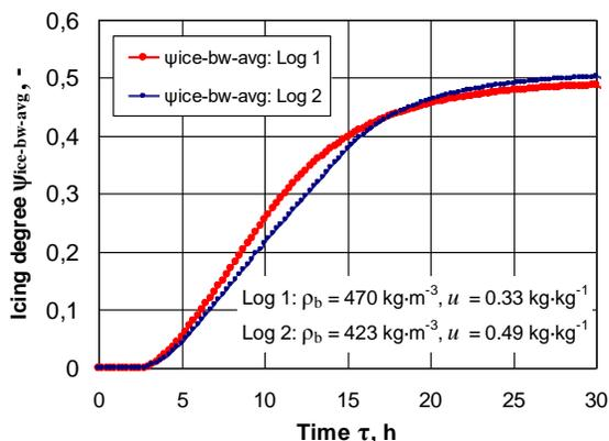
Figure 4. Change in  $\Psi_{ice-bw-avg}$  during the freezing of the studied pine logs
