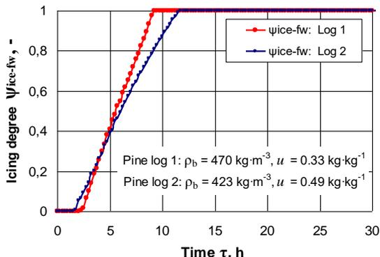
Figure 3. Change in  $\Psi_{ice-fw}$  during the freezing of the studied pine logs
