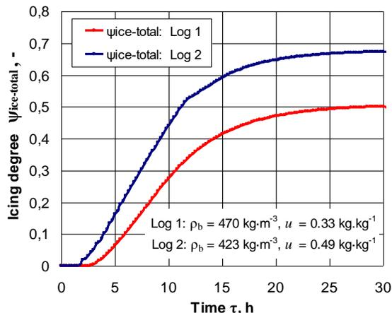
Figure 5. Change in  $\Psi_{ice-total}$  during the freezing of the studied pine logs
