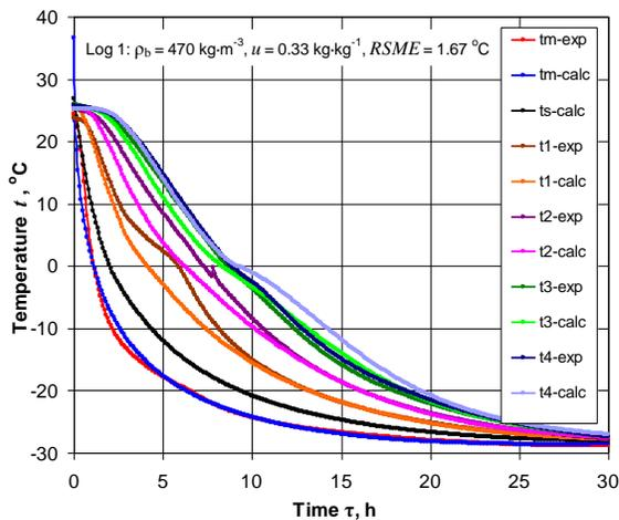
**Figure 1.** Calculated and experimentally determined change in  $t_m$ ,  $t_s$ , and  $t$  in 4 points of the Log 1 during its 30 h freezing
